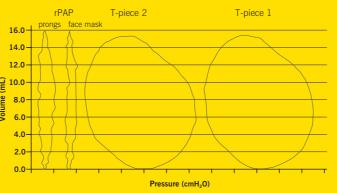
I T-piece 1 I rPAP with prongs I T-piece 2 I rPAP with face mask
