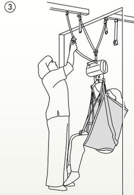
Then attach the lift strap to the Quick-Release Hook in room 2 and run in the lift strap. The patient is now transferred to room 2.
