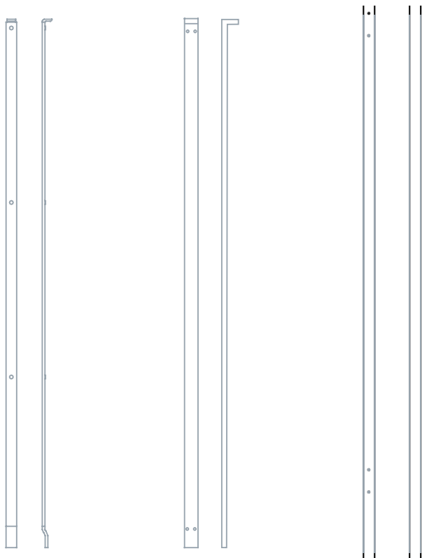
Slimline Upright Support: Max Load 272 kg / 600 lbs
